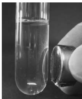
Figure 2. Separation of Cs2.5-APS/Fe x O y @SiO 2 from an aqueous solution containing ethyl acetate using an external magnet.
